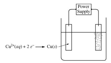
3. An external direct-current power supply is connected to two platinum electrodes immersed in a beaker containing  $1.0 \, M \, \text{CuSO}_4(aq)$  at  $25^{\circ}\text{C}$ , as shown in the diagram above. As the cell operates, copper metal is deposited onto one electrode and  $O_2(g)$  is produced at the other electrode. The two reduction half-reactions for the overall reaction that occurs in the cell are shown in the table below.
